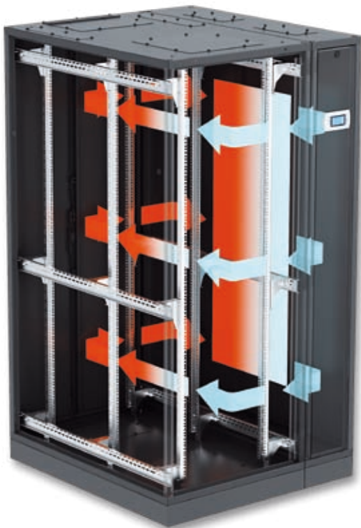
Server cabinet with a side heat exchanger. Cabinet width: 800 mm, heat exchanger width: 300 mm. Cabinet door with mineral safety glass
