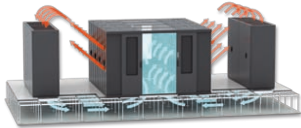
Server room cooling in the "cold aisle" technology with using access floor
