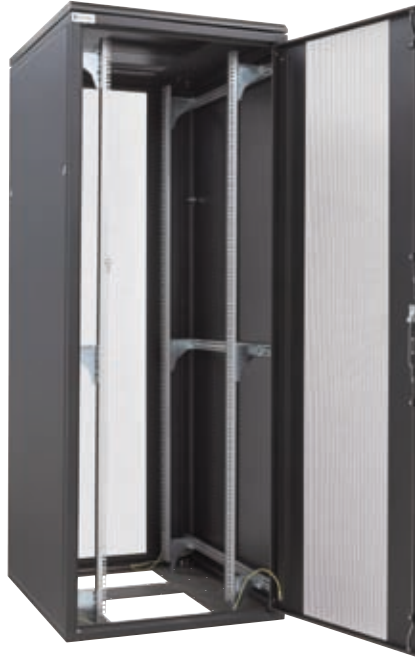
Cabinet SZB SE 42 U, 800x1000 mm, colour: RAL 9005, set on levelling feet, door with perforation type C, two pairs of mounting profiles in 19" spacing Catalogue no. WZ-SZBSE-005-5711-11-0000-2-161
