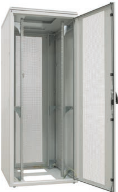
OTS1 cabinet 42 U, 800 x 1000 mm with perforated steel doors and three-point rod-latch locks with swing handle
