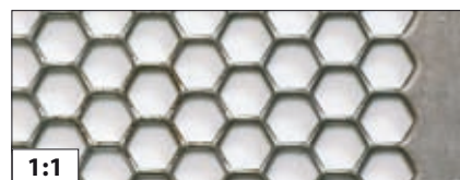
Perforation type C clearance 80%
