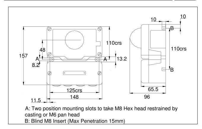
Figure 2 Direct Surface mounting (in mm)
