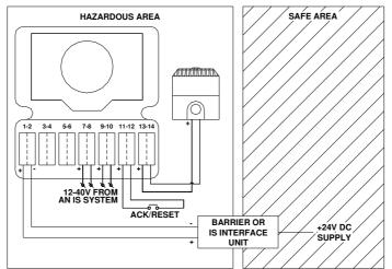
Figure 8 DA135 connected as single point annunciator with sounder.
