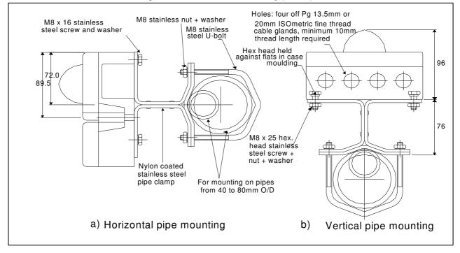
Figure 3 Pipe/post mounting (in mm)
