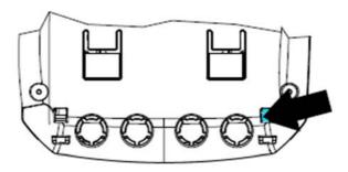
Leave a gap at least 0.8 cm wide between the sensor and installation wall. Do not place the sensor near objects that could heat and alter temperature readings.
